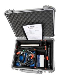
Continuous proximity CP and electrical Field Gradient (FG) readings can be read simultaneously coupled with contact measurement when required without having to change setting or probes.
